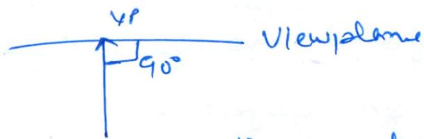
Orthographics projection is the projection on one of the co-ordinate planes i.e.  $x=0, y=0, z=0$ .
